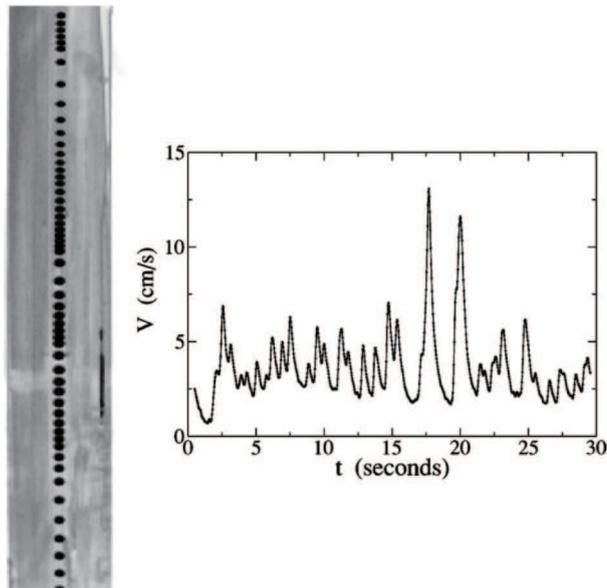
Figure 1 Oscillations of a solid ball falling through a wormlike micellar fluid.
