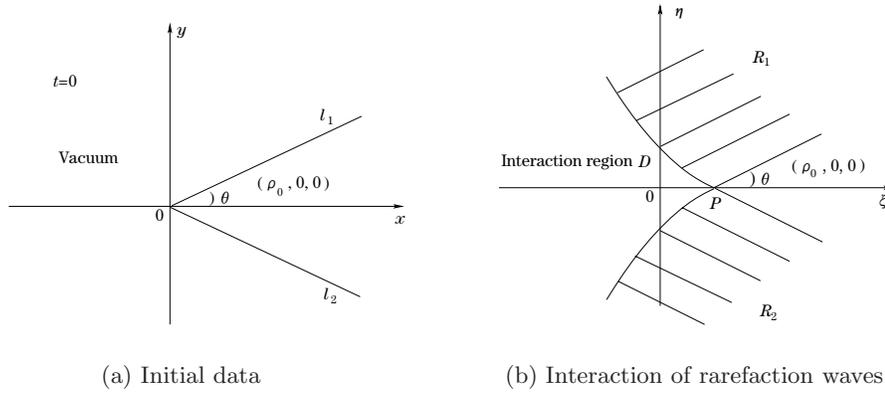
Figure 3.1 The expansion of a wedge of gas
